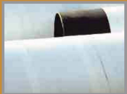
Finally, the coating is quickly cut back at the ends before bonding is permanent.
